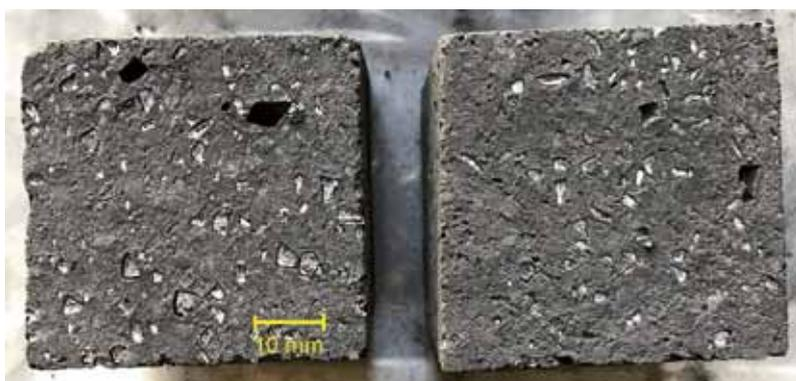
**Fig. 2** Digital micrograph of the surface of sample M1
