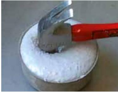
**Fig. 12** Microsilica castable: hammer penetrating the castable, approx. 0,03 s after impact, no signs of dilatancy
