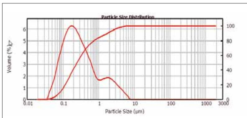
**Fig. 5** Typical PSD of microalumina
