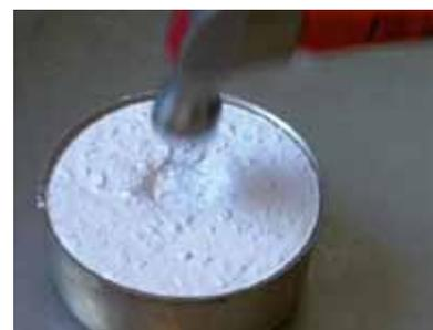
**Fig. 11 Alumina castable:** approx. 0,25 s after impact; hammer bouncing back; due to dilatancy just a shallow indentation from the hammer blow is observed, no penetration
