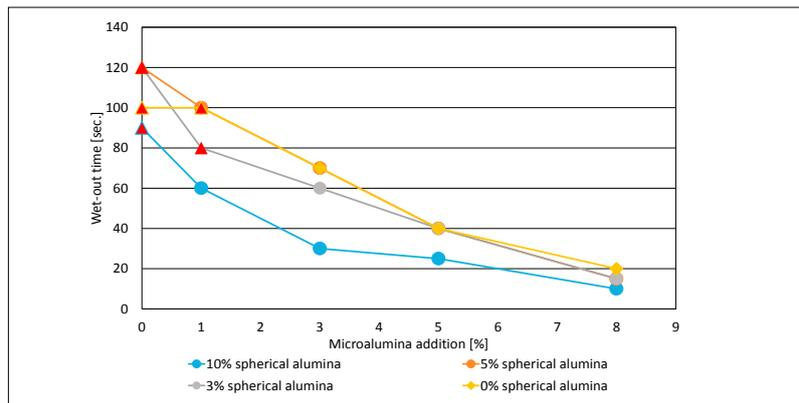
**Fig. 16** Wet-out time for the corundum-spinel castables as a function of content of spherical particles: there is a profound effect on wet-out by replacing reactive alumina with microalumina. Also, dilatancy is influenced heavily. Red triangles are indicative of casting difficulties, like dilatancy; hence, the castables without microalumina additions (those indicated with red triangles) can in practise not be made at the current water addition level
