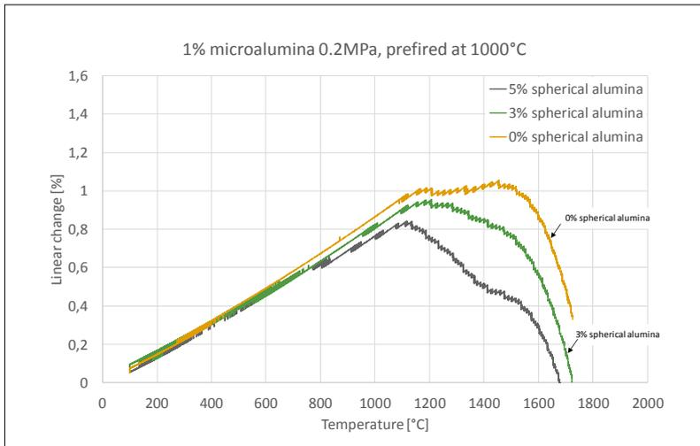
**Fig. 18** RUL of alumina–MgO samples with 1 % microalumina pre-fired at 1000 °C prior to testing; samples with 0, 3 or 5 % spherical alumina respectively
