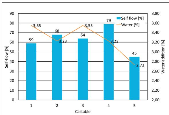
**Fig. 14** Flow, porosity and water addition for the castables in Tab. 2
