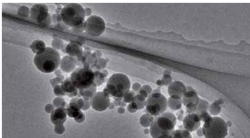
**Fig. 2** Elkem Microsilica 971, TEM micrograph
