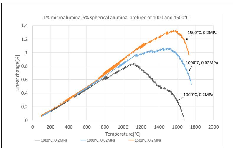
**Fig. 20** RUL of alumina–MgO samples with 1 % microalumina pre-fired at 1000 °C, and 1500 °C prior to testing; load 0,2 MPa and 0,02 MPa; samples with 5 % spherical alumina
