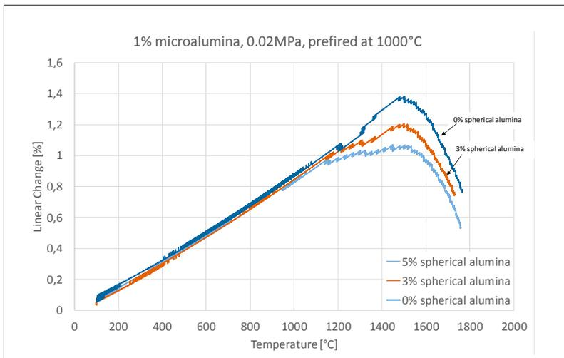
**Fig. 19** Assisted sintering of alumina–MgO samples pre-fired at 1000 °C prior to testing; samples with 0,3 or 5 % spherical alumina respectively, and 1 % microalumina
