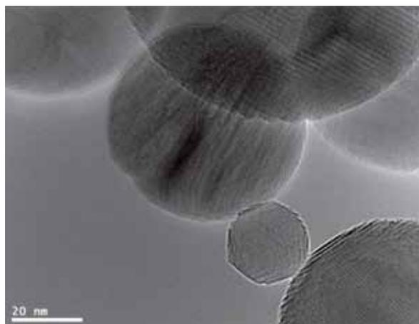
**Fig. 4** Microalumina close-up: at a closer view some of the “spherical” crystals show the beginning of faceting; the curved surfaces show small steps
