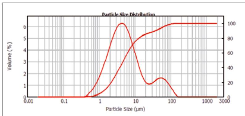
**Fig. 6** Typical PSD of spherical alumina
