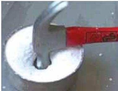
**Fig. 13** Microalumina castable: approx. 0,03 s after impact, hammer deeply sunken into the castable, dilatancy is almost non-existent; the castable surface is curved due to high surface tension
