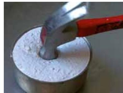
**Fig. 10 Alumina castable:** approx. 0,1 s after impact
