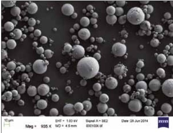
**Fig. 7 Spherical alumina:** this alumina quality contains both small and larger spheres
