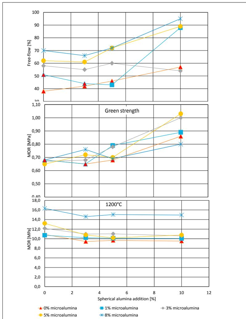
**Fig. 17** Flow, green-strength (MOR), and Hot-MOR after 24 h firing at 1200 °C of the CC corundum-spinel castables, showing the effect of spherical particles on self-flow and the improvement of the green strength by the replacement of calcined alumina by spherical alumina
