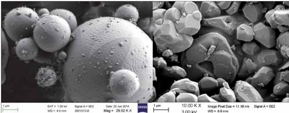
**Fig. 21** Comparison of spherical alumina and calcined alumina at approximately same magnification (bar = 1 µm)
