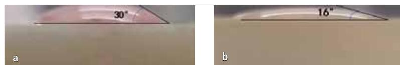
**Fig. 1 a–b** Wetting angles of simulated molten slag and (a) alumina disc, (b) resin disc
