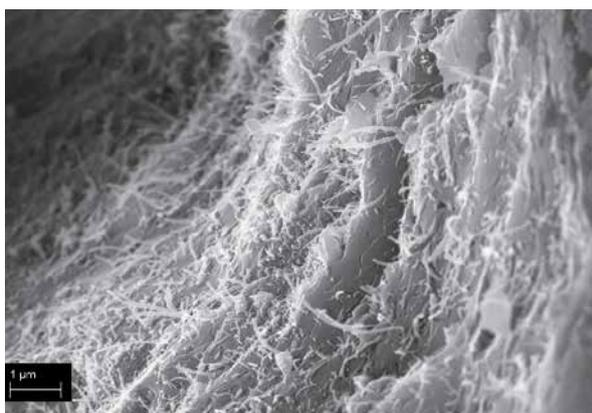
**Fig. 2** Detail of a CNF agglomerate in a CNF doped coal-tar pitch fracture surface
