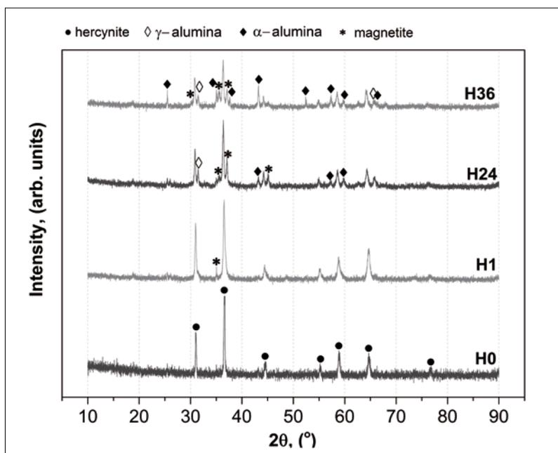
**Fig. 1** XRD patterns for the as-synthesized sample of hercynite ( $H_0$ ) and the after-annealing ones ( $H_1$ ,  $H_{24}$  and  $H_{36}$ )
