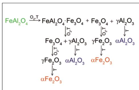
**Fig. 8** Model of hercynite decomposition in air
