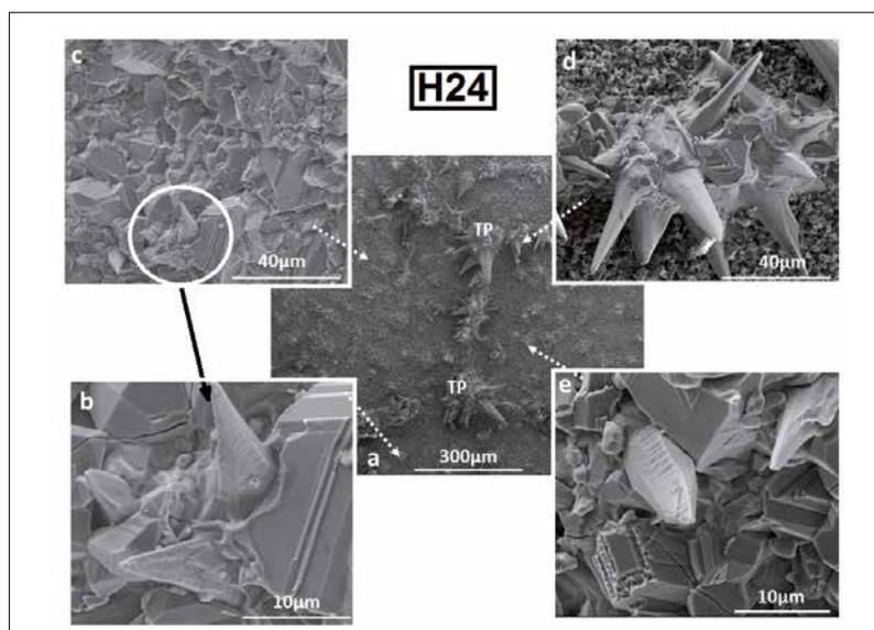
**Fig. 5 a–e** Microstructure of hercynite sample after 24 h thermal treatment at 1000 °C ( $H_{24}$ )
