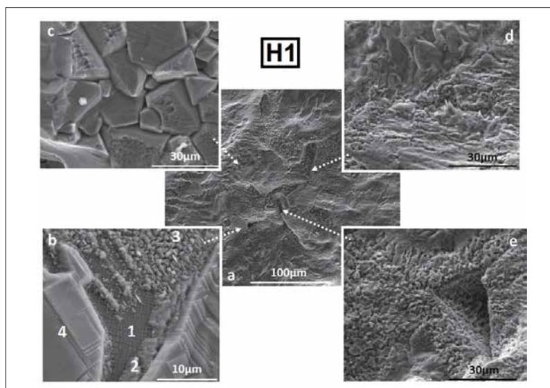
**Fig. 4** Microstructure of hercynite sample after 1 h thermal treatment at 1000 °C ( $H_1$ )
