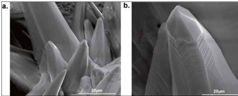
**Fig. 6** Microstructure of hercynite sample after 36 h thermal annealing at 1000 °C ( $H_{36}$ )
