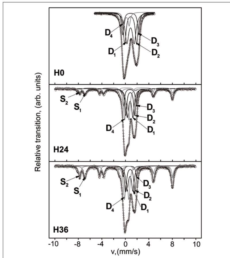
**Fig. 2** Mössbauer spectra for the as-synthesized sample of hercynite ( $H_0$ ), and the samples after thermal annealing ( $H_{24}$  and  $H_{36}$ )
