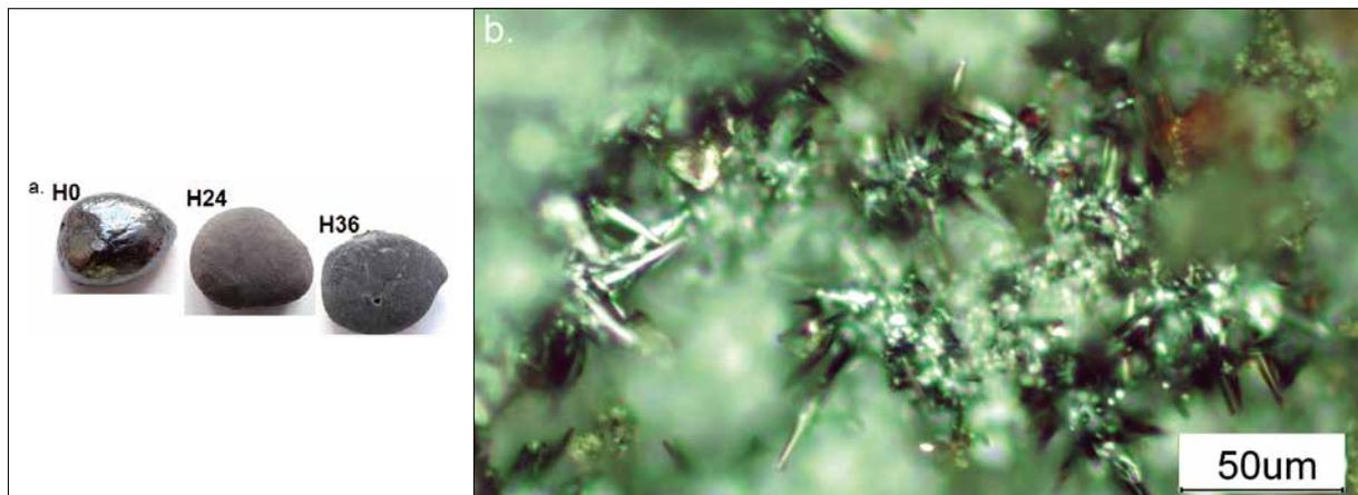
**Fig. 3 a–b** a) Macrostructure of the as-synthesized sample ( $H_0$ ), and the samples after thermal annealing  $H_{24}$  and  $H_{36}$  sample; b) microstructure of the surface of  $H_{36}$  sample
