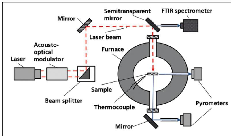
**Fig. 4** Schematic sketch of TOM\_wave together with the laser beam path during laser-flash measuring
