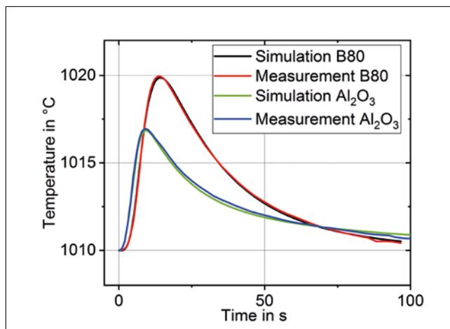
**Fig. 6** Laser-flash measuring of an alumina and a bauxite (B80) sample: comparison of measured and simulated temperature curves
