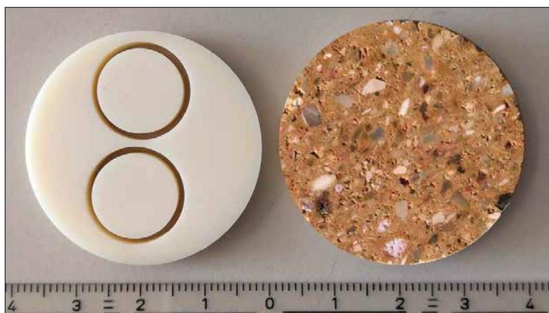
**Fig. 7** Used samples: alumina disk with two smaller samples extracted for the comparison with LFA457 measurement (l.), and bauxite disk extracted from a refractory brick (r.)
