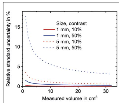
**Fig. 1** Effect of measuring volume, characteristic size of constituting phases, and material contrast on variation of resulting material property
