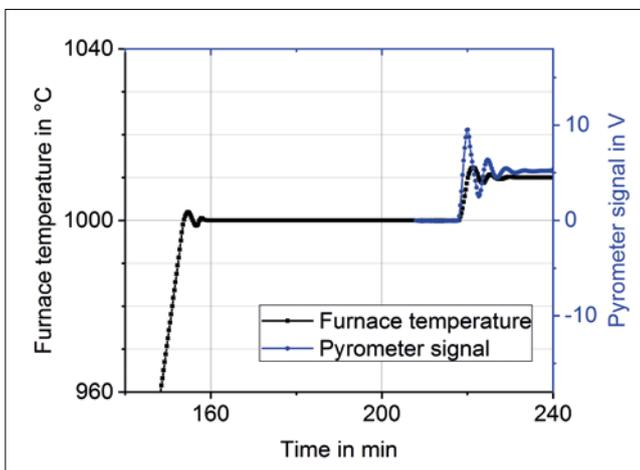
**Fig. 5** Temperature profile during a holding period with subsequent step heating
