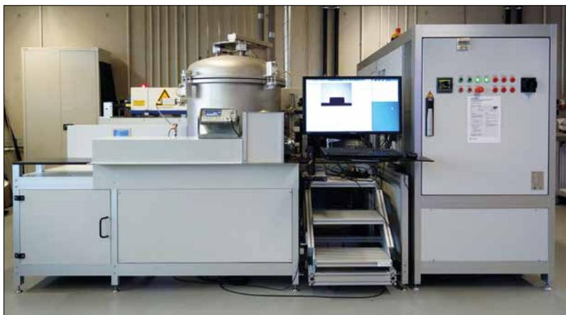
**Fig. 2** Photograph of the thermo-optical measuring device TOM\_wave showing the upper part of the high temperature furnace, and – in the background – the CO<sub>2</sub> laser
