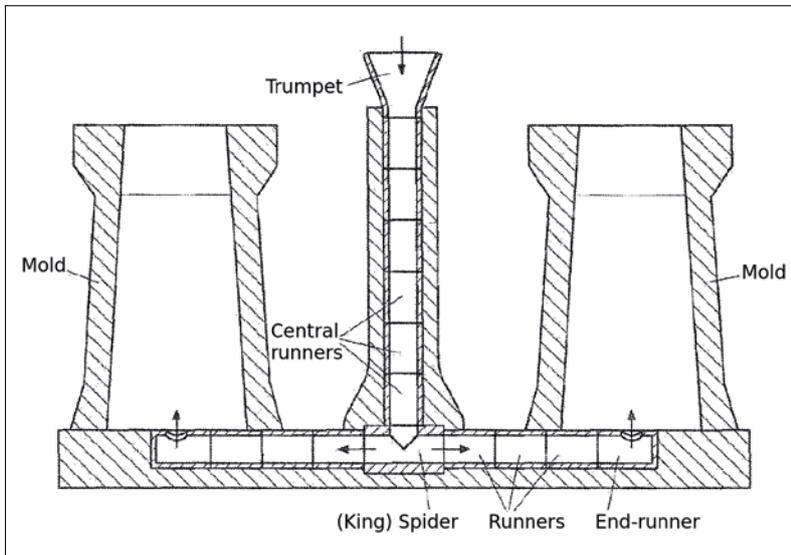
**Fig. 2 Exemplary refractory pipe system used in bottom teemed steel ingot casting after Ritter et al. [6, Fig. 1]**
