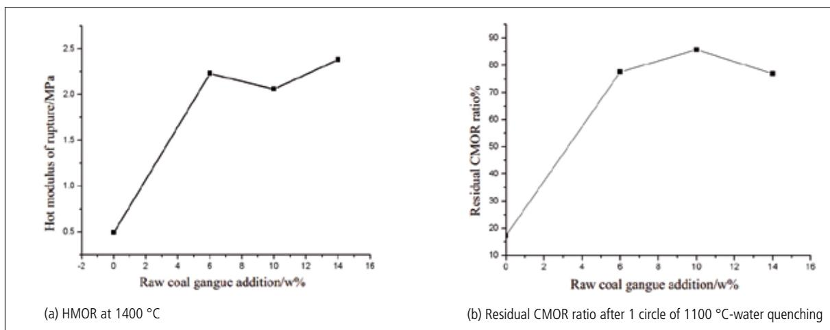
**Fig. 4** Effects of adding coal gangue (up to 14 mass-%) in LC Al<sub>2</sub>O<sub>3</sub>-SiO<sub>2</sub> castables
