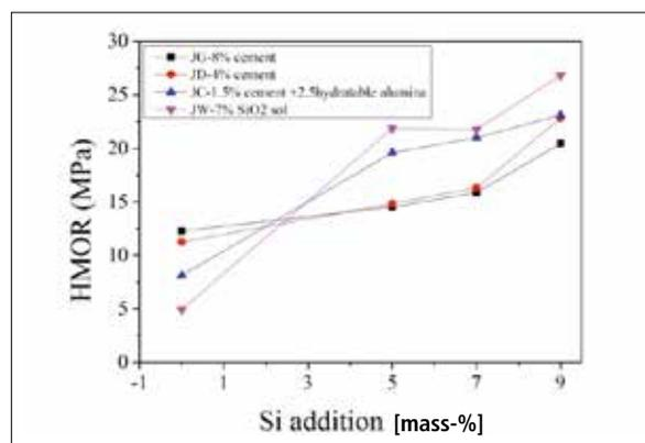
**Fig. 2** HMOR of high alumina castables incorporated with Si powder after nitridation (4 binding systems: high level of cement, low cement, ultra low cement and non-cement; pre-treatment: nitridation at 1450 °C for 9 h; test: 1300 °C, 0,5 h, carbon embedded)
