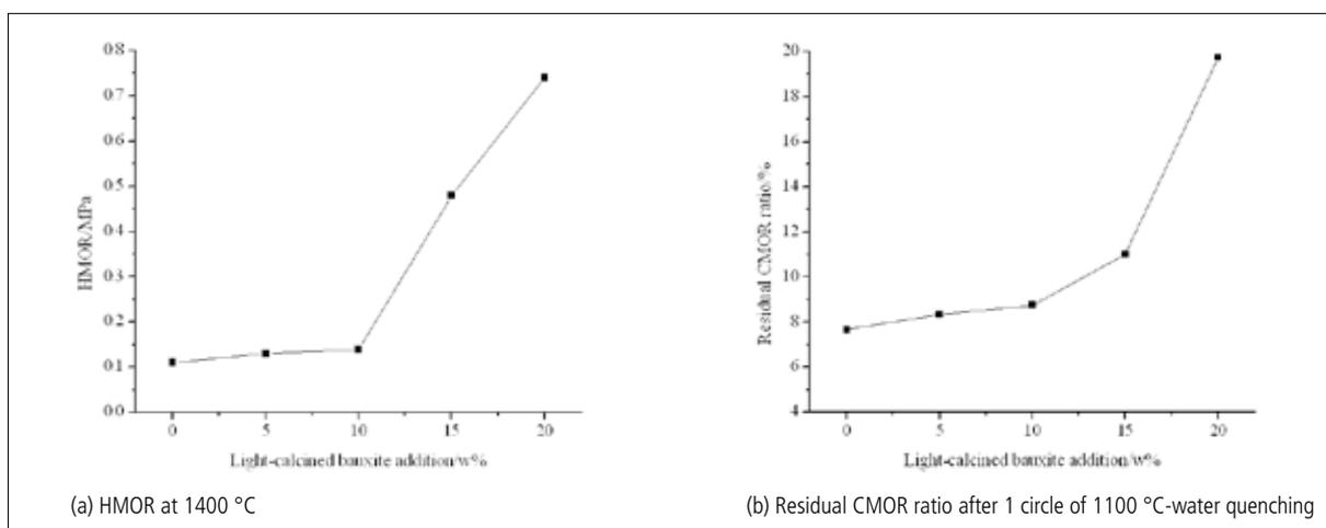
**Fig. 5** Effects of adding mild-calcined bauxite (up to 20 mass-%) in LC Al<sub>2</sub>O<sub>3</sub>-SiO<sub>2</sub> castables
