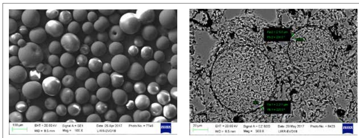
**Fig. 10** Stress dissipative aggregates of alumina micrograins, as-received and in the castable
