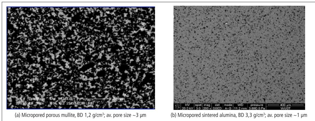
**Fig. 11** Micropored porous and dense aggregates
