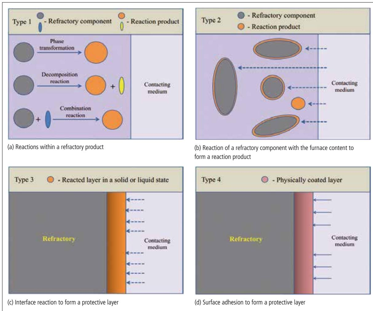
**Fig. 3** Four types of in situ refractory
