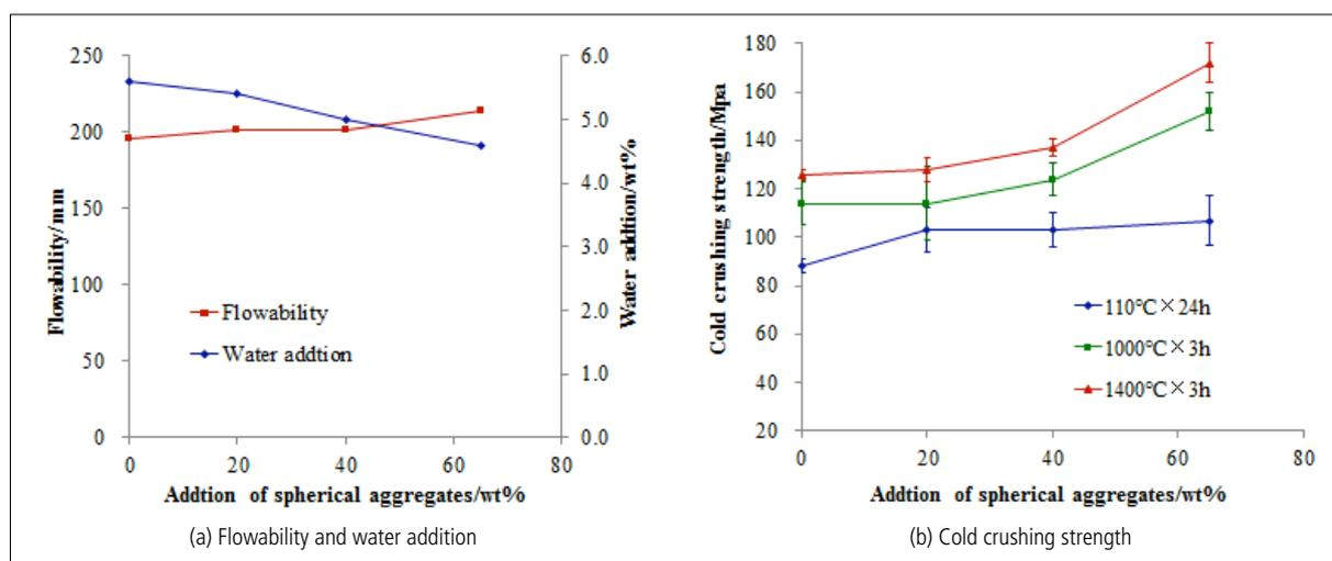
**Fig. 9** Properties comparison of Al<sub>2</sub>O<sub>3</sub>-SiO<sub>2</sub> castables using spherical bauxite to replace conventional bauxite aggregates
