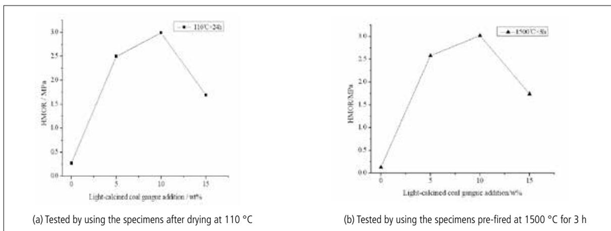
**Fig. 6** HMOR at 1400 °C of the Al<sub>2</sub>O<sub>3</sub>-SiO<sub>2</sub> castables with mild-calcined coal gangue (up to 15 mass-%), using specimens with and without pre-firing respectively
