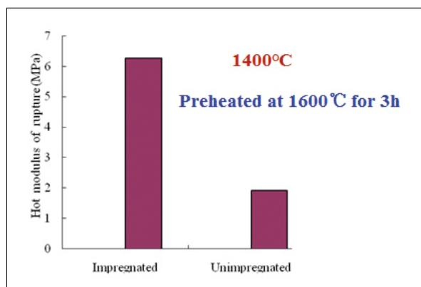
**Fig. 1** Effect of impregnation with a magnesium sulphate solution on HMOR of an  $\text{Al}_2\text{O}_3$  based castable
