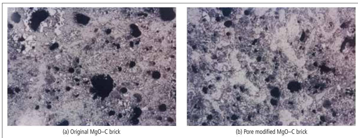
**Fig. 12** Microstructure comparison between the MgO-C bricks with and without using pore-modifying additive
