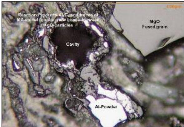
**Fig. 2** Microphoto of an MgO-C brick containing 2 % Al-powder after 1000 °C in reducing atmosphere
