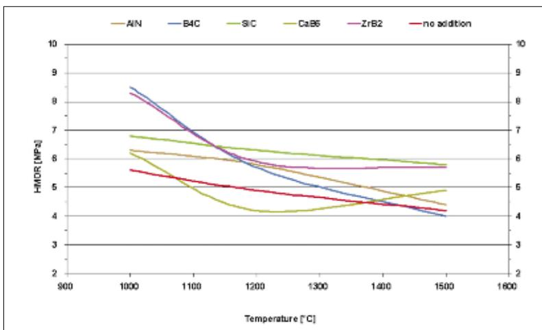
**Fig. 5** Influence of non-metallic antioxidants on the HMOR of MgO-C bricks
