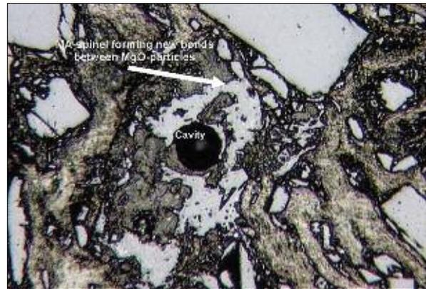
**Fig. 3** Microphoto of an MgO-C brick containing 2 % Al-powder after 1500 °C in reducing atmosphere
