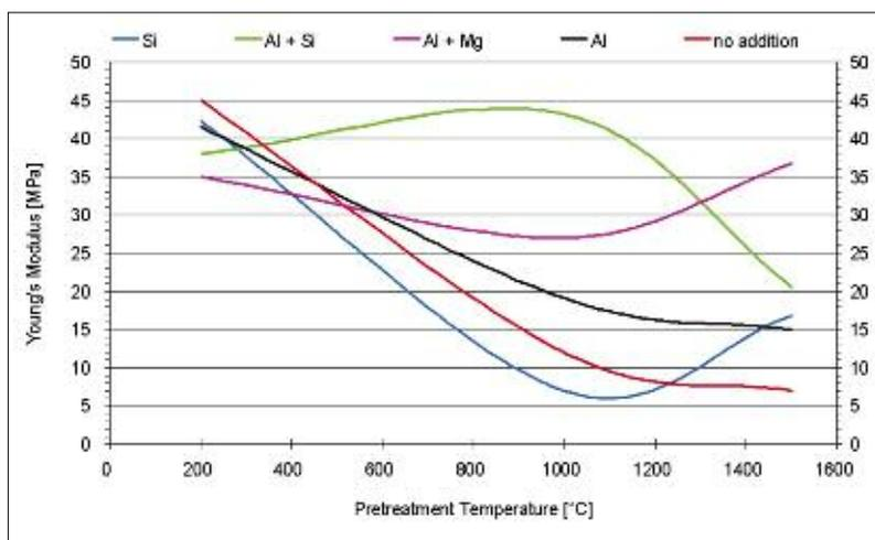
**Fig. 6** Influence of metallic antioxidants on the Young's modulus of MgO-C bricks, pretreated at different temperatures
