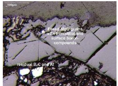
**Fig. 11 Dense layer of an MgO-C brick with an addition of  $B_4C$  and Al-powder**
