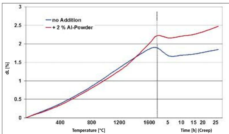
**Fig. 7** RUL and creep of MgO-C bricks with and without 2 % Al
