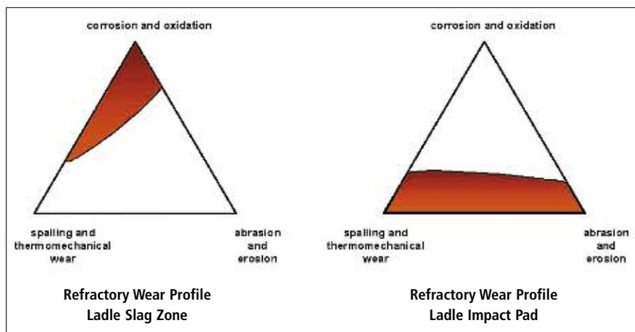
**Fig. 14** Refractory wear in a ladle
