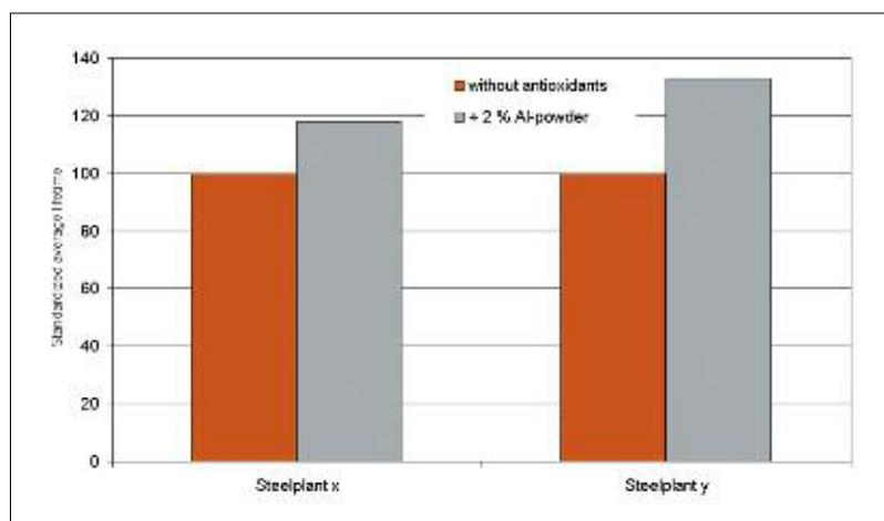
**Fig. 15** Performance in ladle bottom impact pads; Al<sub>2</sub>O<sub>3</sub>-MgO-C brick, BFA-basis, 5 % C
