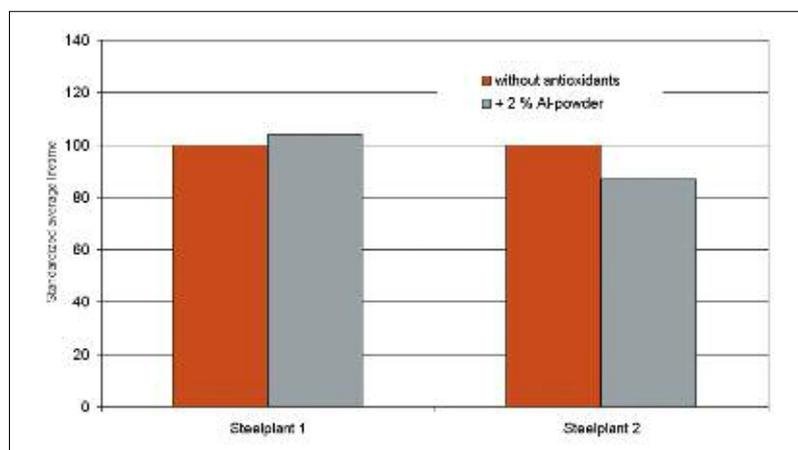
**Fig. 16** Performance in ladle slag lines; MgO-C brick, 98 FM-basis, 15 % C
