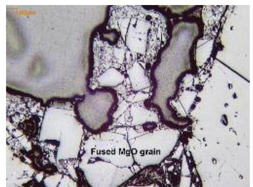
**Fig. 12 Microphoto of brick type 2 after 46 heats service in a steel ladle slag line**
