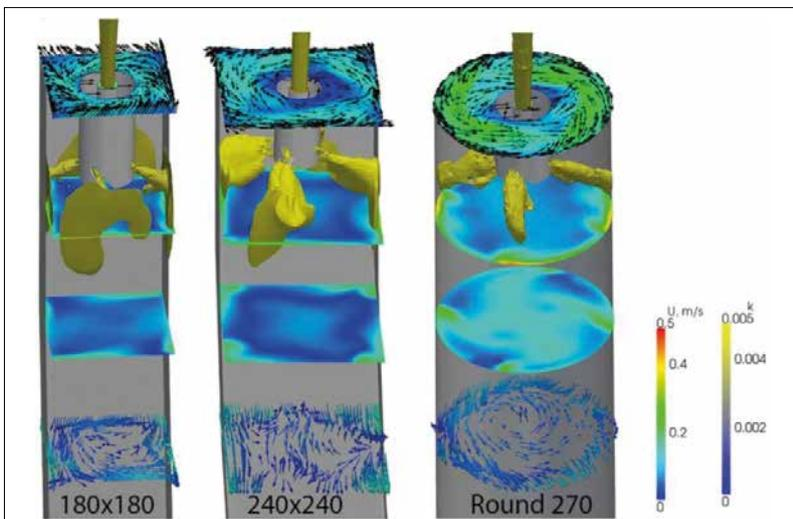
**Fig. 3** Velocity profile of the meniscus using the GYRONOZZLE for different mould sizes
