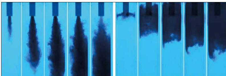
**Fig. 2** Comparison of the jet penetration by using a single-hole nozzle (l.) , and the GYRONOZZLE (r.) by using a water model with dye injection
