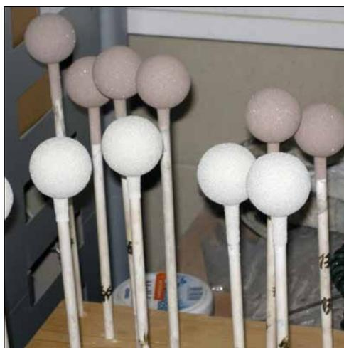
**Fig. 8** Shelled ping pong balls for determining the permeability of the shell
