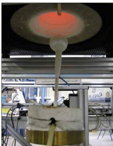
**Fig. 9** Furnace for measuring the hot permeability
