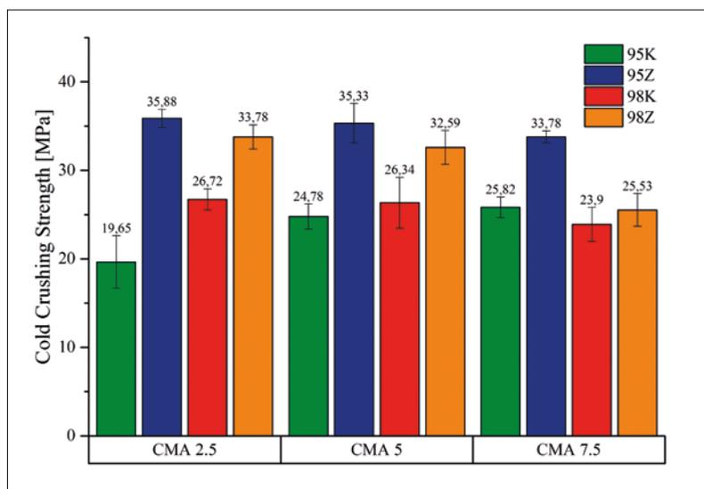
**Fig. 1** CCS of samples containing SM 98 and CS 95, respectively, as well as MagA aggregates and powder, respectively
