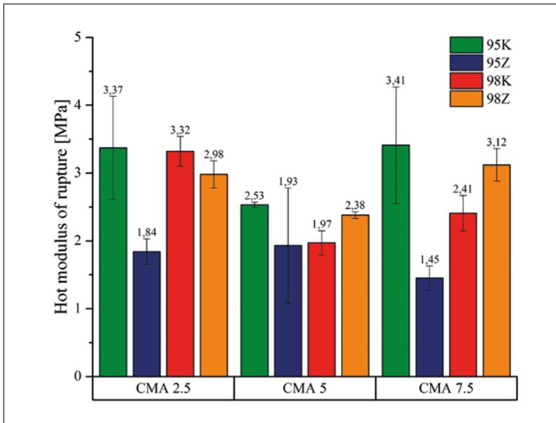
**Fig. 2** HMOR of samples containing SM 98 and CS 95, respectively, as well as MagA aggregates and powder, respectively
