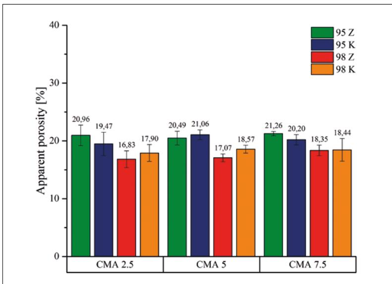
**Fig. 3** Apparent porosity of samples containing SM 98 and CS 95, respectively, as well as MagA aggregates and powder, respectively
