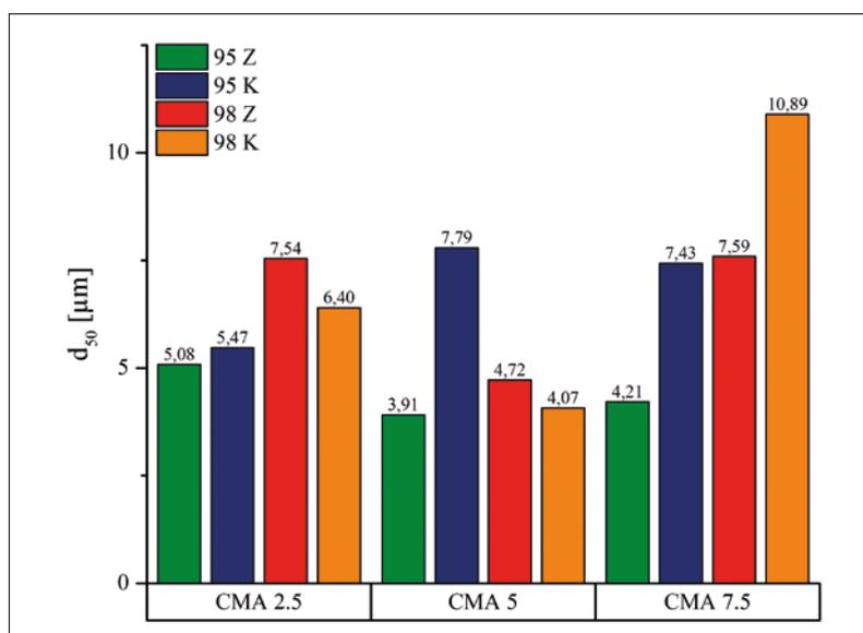
**Fig. 4** The  $d_{50}$  value of samples containing SM 98 and CS 95, respectively, as well as MagA aggregates and powder, respectively
