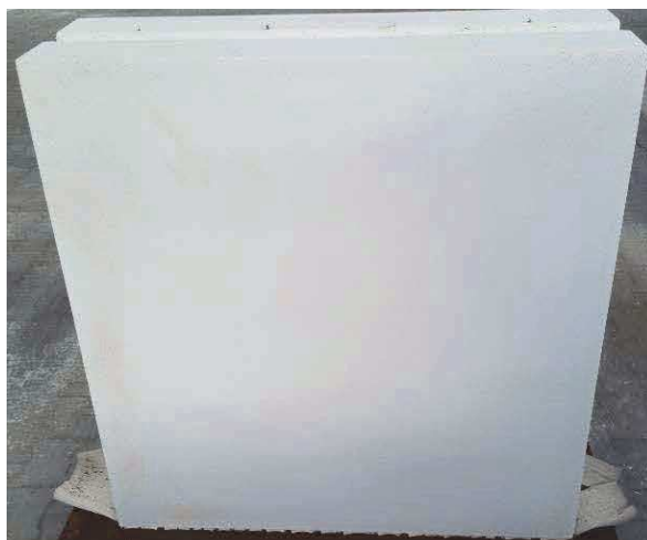
Fig. 12 950 kg HYBRID sample after rapid heating up to 500 °C
