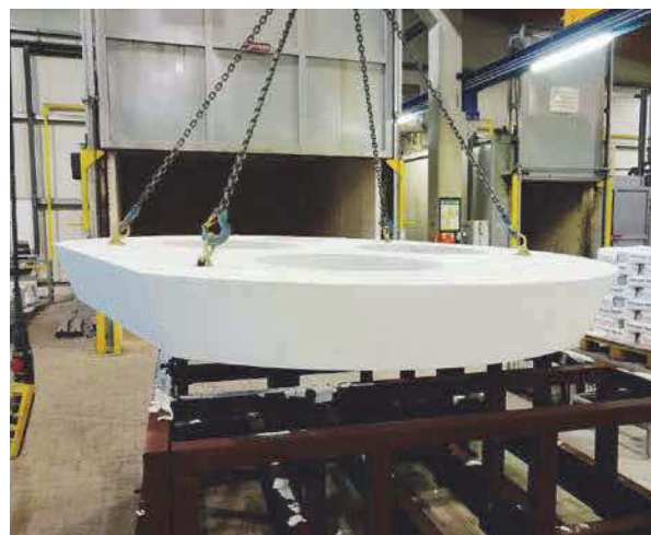
Fig. 13 EAF cover plate, made of REFRACAST® HYBRID A-72 CT/S, dried and demoulded without damages, lifted at only four anchor points after curing
