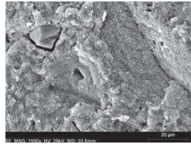
Fig. 7 SEM picture (1500 ×) of HYBRID fractured surface, modified gelation with crystalline structure
