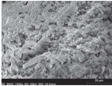
Fig. 5 SEM picture (1500 ×) of LCC fractured surface, bright hydrate phases visible
