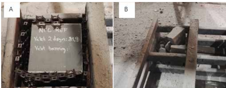
Fig. 3 ~80 kg block (A) before and (B) after explosion resistance test (from 20–850 °C at 50 °C/h)
