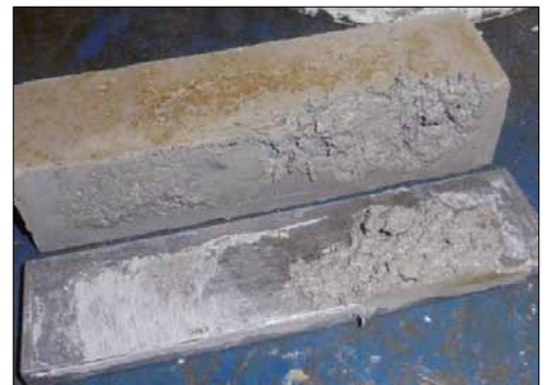
Fig. 3 Castable with dispersant C after curing for two days at 20 °C
