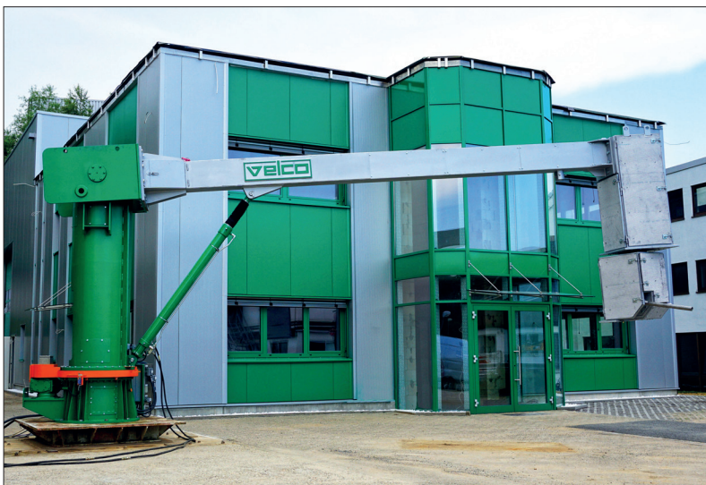
Fig. 3 Gunning robot Hytop near the company’s new building
